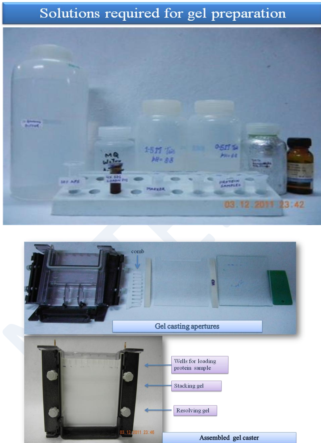
Figure 2B: Experimental set-up and requirements for a polyacrylamide gel electrophoresis
